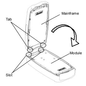
Figure 2.11-1 Alignment Tabs and Slots
