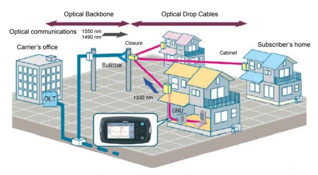
Figure 1.2-1 Finding Faults in Fiber from Each Subscriber's Home (Passive Optical Network Measurement)
