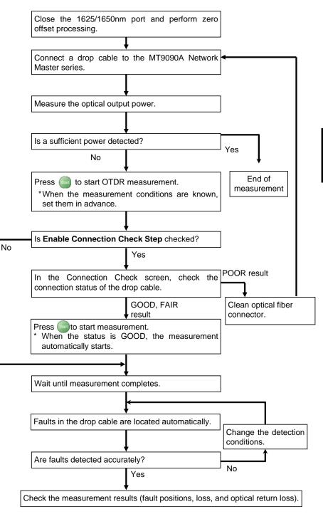
Figure 5.2-1 Drop Cable Measurement Procedure
