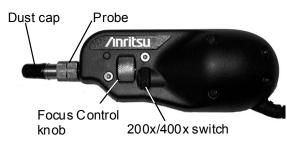
Figure 9.1-2 Video Inspection Probe (VIP)
