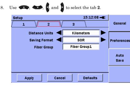
Figure 3.3.2-2 Setup-Preferences Screen 2 (In case of OTDR or DCFL function)
