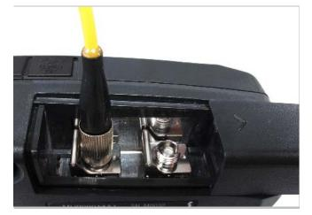
Figure 2.6-1 Connecting Fiber to Measurement Port
