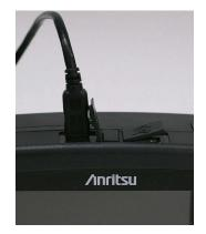
Figure 2.10.2-1 USB Cable Connection
