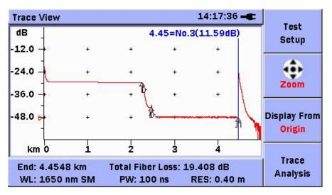
Figure 1.1.1-1 Example of OTDR Measurement Results
