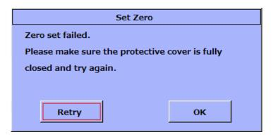
When the set zero is re-executed, confirm the slide cover is firmly closed, and then select **Retry**. Press **set** to start the set zero.
